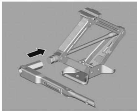
6. Slide the wheel wrench onto the drive nut of the jack.
