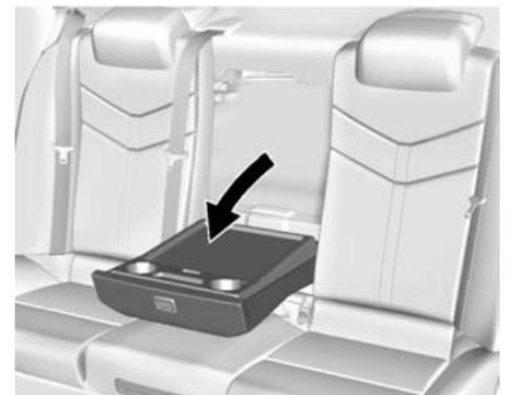
The rear seat has a rear seat pass-through door in the center of the rear seatback. Press the button on top of the seatback and fold the center part of the seatback down to access the trunk. There are two cupholders on the door. To close, lift the pass-through door and push it rearward until it locks into place.
