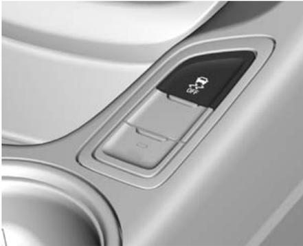
To turn the system off, press the TCS/StabiliTrak button on the center console.
