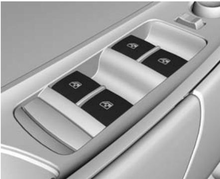
Press the switch down to open the window. Pull the switch up to close it.
