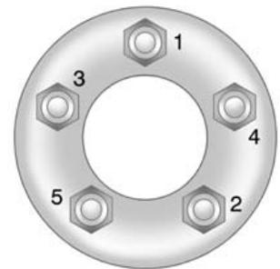
15. Tighten the wheel nuts firmly in a crisscross sequence, as shown.
