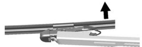
3. Install the new blade onto the arm connector and make sure the tabs are fully set in the locked position.
