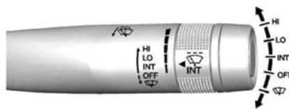
With the ignition in ACC/ACCESSORY or ON/RUN/START, move the windshield wiper lever to select the wiper speed.
