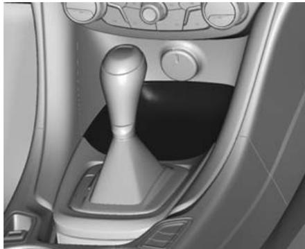
2. Remove the trim from the center console, in front of the shift lever.
