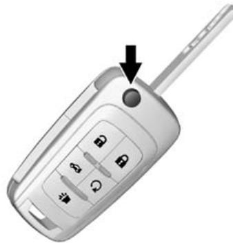
Press the button on the RKE transmitter to extend the key. Press the button to retract the key.
