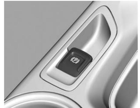
The vehicle has an Electric Parking Brake (EPB). The switch is on the center console. The EPB can always be activated, even if the ignition is off. To prevent draining the battery, avoid repeated cycles of the EPB when the engine is not running.
