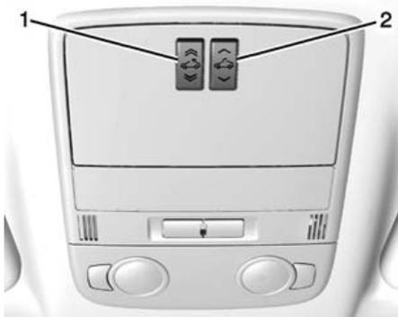
**Open/Close:** Press and hold the front or rear of the switch (1) to open or close the sunroof. The sunshade automatically opens with the sunroof, but must be closed manually.
