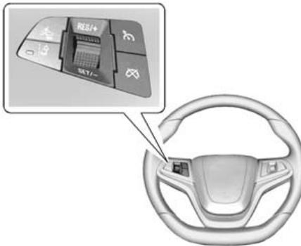
**On/Off:** Press to turn the cruise control system on and off. A white cruise control indicator appears in the instrument cluster.
