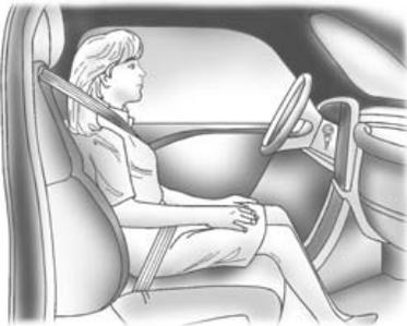
If a person of adult-size is sitting in the front outboard passenger seat, but the off indicator is lit, it could be because that person is not sitting properly in the seat. Use the following steps to allow the system to detect that person and enable the front outboard passenger frontal and knee airbags:
