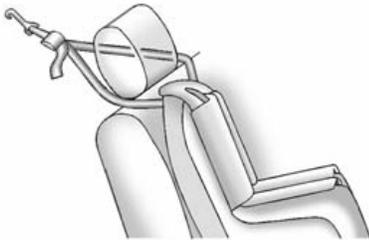
If the position you are using has a fixed head restraint and you are using a dual tether, route the tether around the head restraint.
