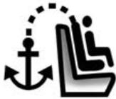
To assist in locating the top tether anchors, the top tether anchor symbol is near the anchor.
