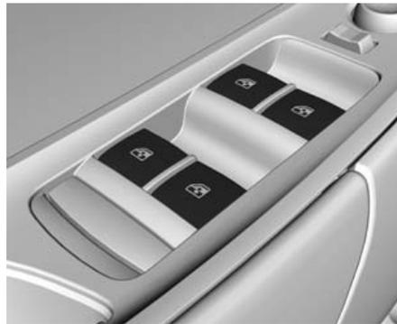
The power window switches on the driver door control all the windows. Each passenger door has a switch that controls only that window.
