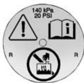
2. Cover the radiator cap with a thick cloth and turn it slowly counterclockwise and remove.
