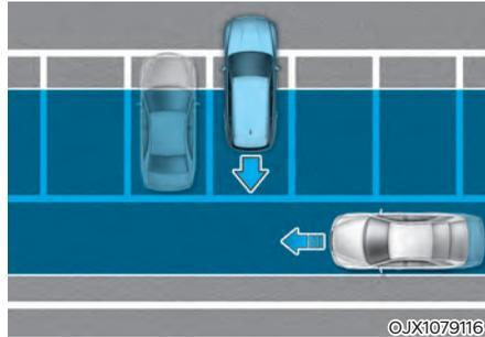
Rear Cross-Traffic Safety system may detect vehicles passing by behind you when parking in reverse into a parking space. If this occurs, the system may unnecessarily warn the driver and control the brake.
