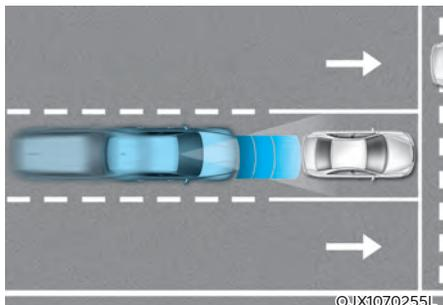
Forward Collision-Avoidance Assist is designed to help detect and monitor the vehicle ahead or help detect a pedestrian or cyclist in the roadway and warn the driver that a collision is imminent with a warning message and an audible warning, and if necessary, apply emergency braking.
