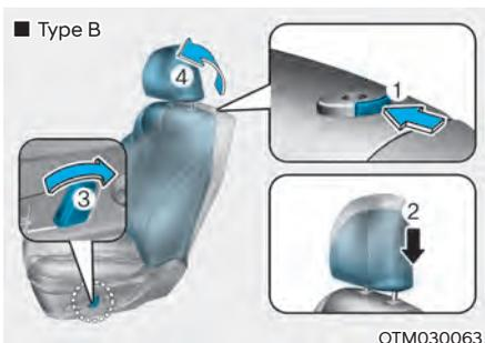
To reinstall the head restraint :
