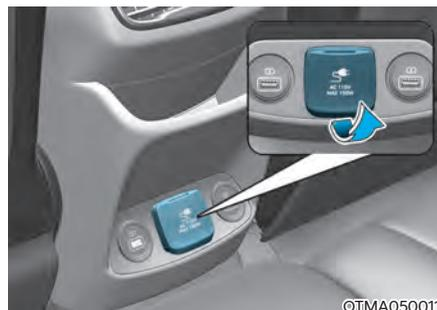
The AC inverter supplies 115V/150W electric power to operate electric accessories or equipments.
