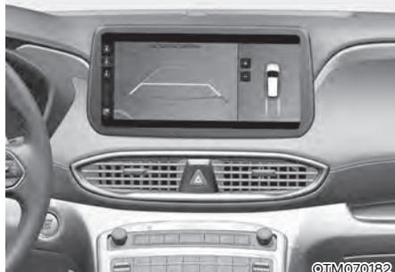
Surround View Monitor can help assist in parking using the cameras installed on the vehicle and displays images around the vehicle through the infotainment system screen.
