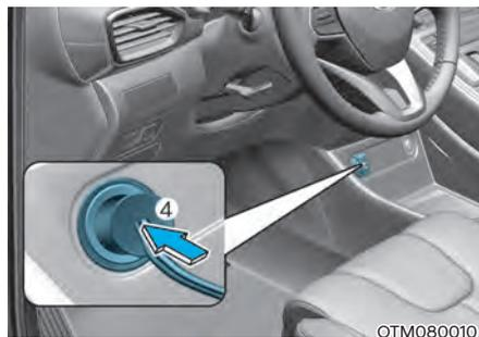
7. Connect the cable and connector (4) to the power outlet in the vehicle.
