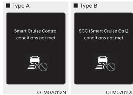
If the Driving Assist button, + switch, - switch or
