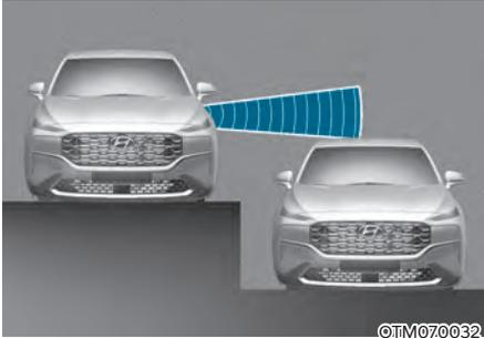
Blind-Spot Safety system may not operate properly when driving where the heights of the lanes are different. The system may not detect the vehicle on a road with different lane heights (underpass joining section, grade separated intersections, etc.).
