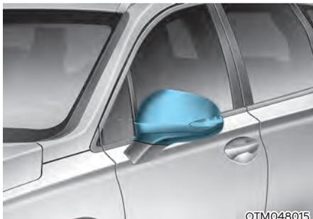
Your vehicle is equipped with both left-hand and right-hand side view mirrors. The mirrors can be adjusted remotely with the mirror adjustment control switch. The side view mirrors can be folded to help prevent damage when going through an automatic car wash or when passing through a narrow street.
