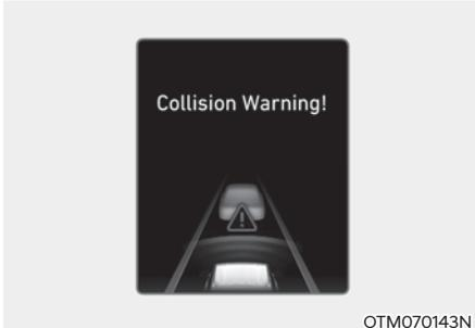
While Smart Cruise Control is operating, when the collision risk with the vehicle ahead is high, the 'Collision Warning' warning message will appear on the cluster, and an audible warning will sound to warn the driver. Always have your eyes on the road while driving, and if necessary, depress the brake pedal to reduce your driving speed in order to maintain a safe distance.
