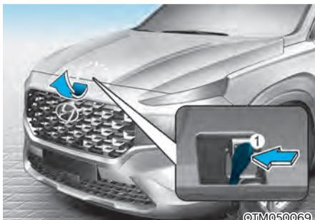
3. Go to the front of the vehicle, raise the hood slightly, push up the secondary latch (1) inside of the hood center and lift the hood.
