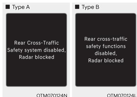
When the rear bumper around the rear-side radar or sensor is covered with foreign material, such as snow or rain, or installing a trailer or carrier, it can reduce the detecting performance and temporarily limit or disable Rear Cross-Traffic Safety system.
