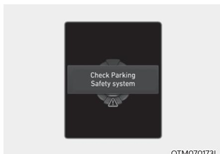
When Reverse Parking Collision-Avoidance Assist or other related systems are not working properly, the 'Check Parking Safety system' warning message will appear on the cluster, and the system will turn off automatically. We recommend that the system be inspected by an authorized HYUNDAI dealer.
