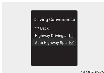
With the engine on, select 'Driver Assistance → Driving Convenience → Auto Highway Speed Control (or Auto motorway speed control)' from the Settings menu to turn on Navigation-based Smart Cruise Control and deselect to turn off the system.
