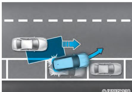
When you are driving forward out of a parking space, if the system judges that there is a collision risk with an approaching vehicle in the blind spot, the system will help avoid a collision by applying the brake.
