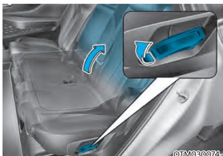
5. To use the rear seat, lift and pull the seatback backward by pulling the folding lever or the strap. Pull the seatback firmly until it clicks into place. Make sure the seatback is locked in place.
