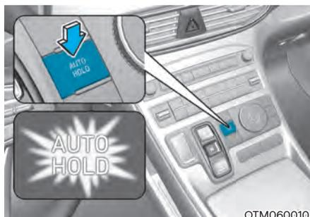
1. With the driver's door, engine hood and liftgate (vehicle equipped with shift button) closed, then press the AUTO HOLD switch. The white AUTO HOLD indicator will come on and the system will be in the standby position.
