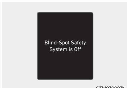
When the engine is restarted with the system off, the 'Blind-Spot Safety System is Off' message will appear on the cluster.
