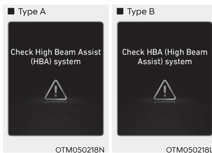
When High Beam Assist is not working properly, the 'Check High Beam Assist (HBA) system' or 'Check HBA (High Beam Assist) system' warning message will appear and
