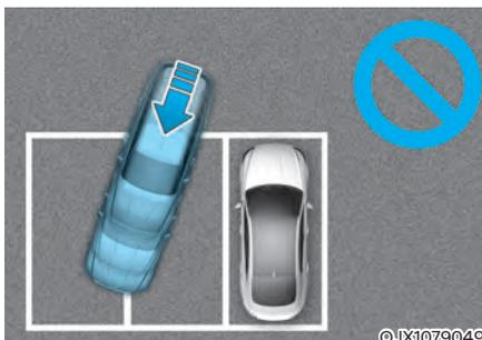
If Remote Smart Parking Assist is used, when parking in a parking space with a vehicle only on one side, your vehicle may cross the parking line to avoid the parked vehicle.
