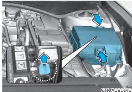
5. Pull the suspected fuse straight out. Use the removal tool (1) provided in the engine compartment fuses panel cover.
