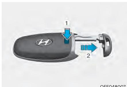
Press and hold the release button (1) and remove the mechanical key (2). Insert the mechanical key into the key hole on the door.
