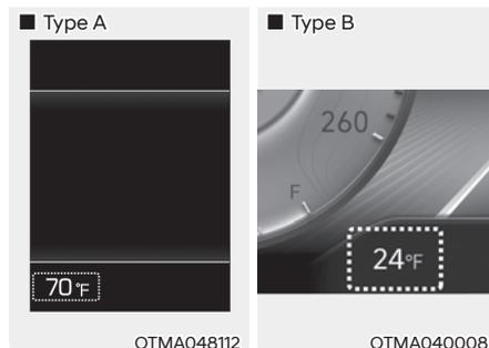
This gauge indicates the current outside air temperatures by 1°F (1°C).
