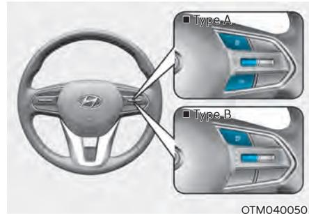
To change the trip mode, toggle the " $\wedge$ ,  $\vee$ " switch on the steering wheel
