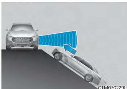
Rear Cross-Traffic Safety system may be limited when the vehicle is on an uphill or downhill slope, or near it, and may not detect the vehicle approaching from the left or right. If this occurs, the system may not warn the driver or control the brakes when necessary.
