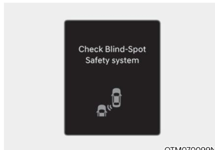
When Safe Exit Assist is not working properly, the 'Check Blind-Spot Safety system(s)' warning message will appear on the cluster, and the system will turn off automatically or the system will be limited. We recommend that the system be inspected by an authorized HYUNDAI dealer.
