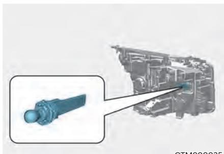
3. Push the wheel guard aside and remove the bulb socket by turning it counterclockwise.
