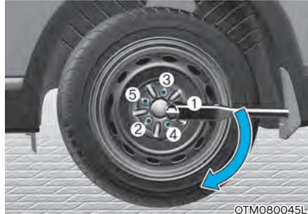
12. Use the wheel lug wrench to tighten the wheel bolts in the order shown. Double-check each wheel bolts until they are tight. After changing tires, we recommend that an authorized HYUNDAI dealer tighten the wheel bolts to their proper torque as soon as possible. **The wheel bolt should be tightened to 79~94 lbf.ft (11~13 kgf.m).**
