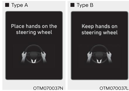
If the driver takes their hands off the steering wheel for several seconds, the 'Place hands on the steering wheel' (or 'Keep hands on the steering wheel') warning message will appear and an audible warning will sound in stages.
