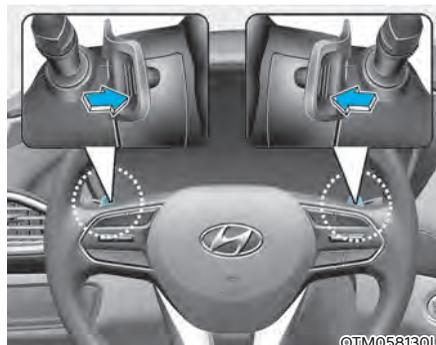
The paddle shifter is available when the shift button is in the D (Drive) position or the manual shift mode.
