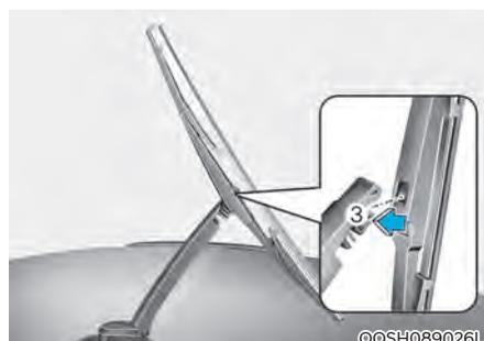
3. Install the new blade assembly by inserting the center part into the slot in the wiper arm until it clicks into place (3).
