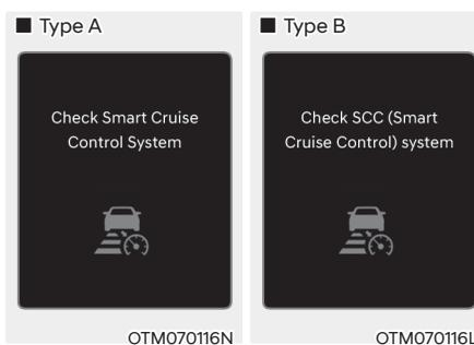
When Smart Cruise Control is not working properly, the 'Check Smart Cruise Control system' (or 'Check SCC (Smart Cruise Control) system') warning message will appear, and the
