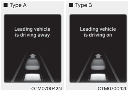
When the front vehicle departs from a stop, Leading Vehicle Departure Alert will inform the driver by displaying the 'Leading vehicle is driving away' (or 'Leading vehicle is driving on') message on the cluster and an audible warning will sound.
