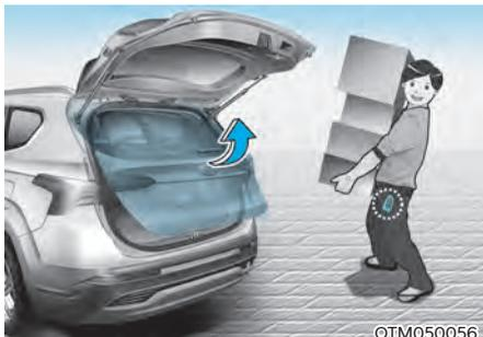
On a vehicle equipped with a smart key, the liftgate can be opened with hands-free activation using the smart liftgate system.
