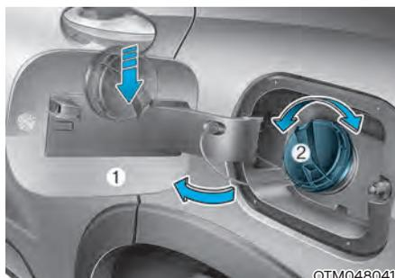
4. Pull the fuel filler door (1) outward to access the fuel tank cap.
