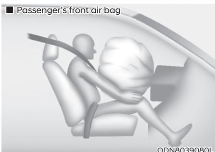
After complete inflation, the air bag immediately starts deflating, enabling the driver to maintain forward visibility and the ability to steer or operate other controls.
