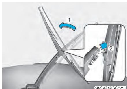
1. Raise the wiper arm and then rotate the wiper blade assembly (1).
