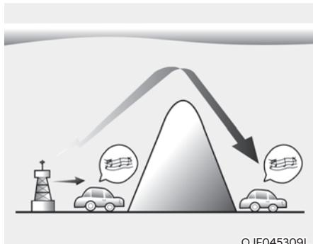
AM broadcasts can be received at greater distances than FM broadcasts. This is because AM radio waves are transmitted at low frequencies. These long, low frequency radio waves can follow the curvature of the earth rather than travelling straight out into the atmosphere.
