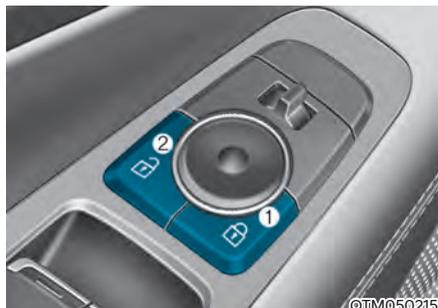
When pressing the (🔒) portion (1) on the switch, all vehicle doors will lock.
