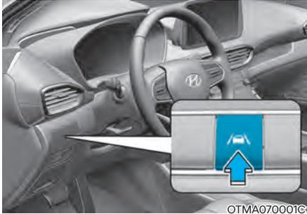
With the engine on, press and hold the Lane Safety button located on the instrument panel to turn on Lane Keeping Assist. The white
