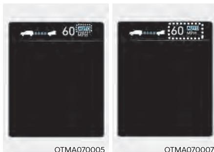
If temporary deceleration is required in the standby state and Navigation-based Smart Cruise Control is operating, the green **AUTO** symbol will illuminate on the cluster.
