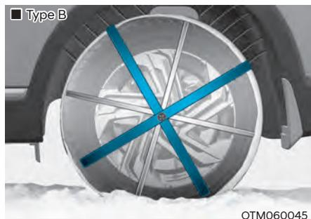
Since the sidewalls of radial tires are thinner than other types of tires, they may be damaged by mounting some types of tire chains on them. Therefore, the use of snow tires is recommended instead of tire chains. If tire chains must be used, use genuine HYUNDAI Parts and install the tire chain after reviewing the instructions provided with the tire chains. Damage to your vehicle caused by improper tire chain use is not covered by your vehicle manufacturer's warranty.
