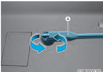
3. Connect the socket and wheel lug nut wrench (A).
