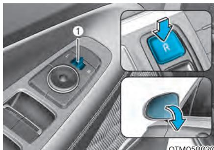
When the gear is shifted to the R (Reverse) position, the side view mirror(s) will rotate downwards to aid with driving in reverse.
