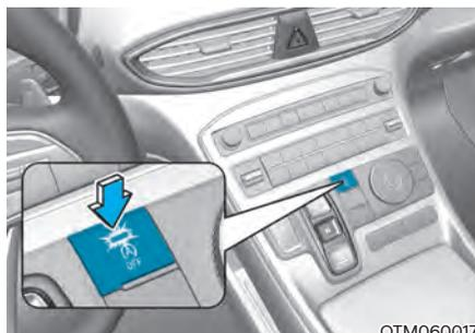
When the system is deactivated, the ISG off button indicator will illuminate and a message 'Auto Stop is off. Shift to P or N to start engine manually' appears on the cluster LCD display with a warning sound.
