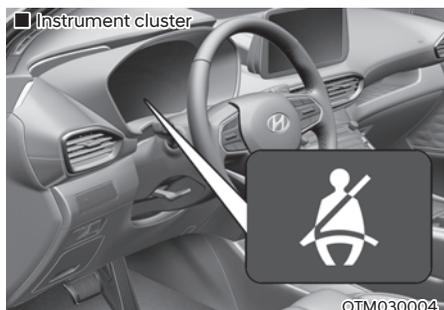
As a reminder to the driver, the seat belt warning light will illuminate for approximately 6 seconds each time you place the ignition switch to the ON position regardless of belt fastening. At this time, if the seat belt is not fastened a warning chime will sound for 6 seconds.
