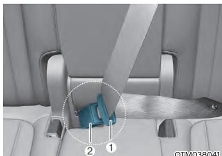
1. Insert the tongue plate (1) into the buckle (2) until an audible “click” is heard, indicating the latch is locked. Make sure the belt is not twisted.
