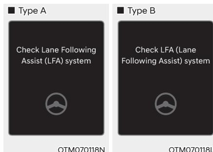
When Lane Following Assist is not working properly, the 'Check Lane Following Assist (LFA) system' (or 'Check LFA (Lane Following Assist) system') warning message will appear on the cluster. If this occurs, we recommend that the system be inspected by an authorized HYUNDAI dealer.
