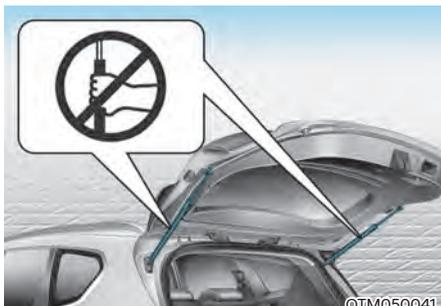
Do not hold the part (gas lifter) that supports the liftgate. Be aware that the deformation of the part may cause vehicle damage and a risk of injury.
