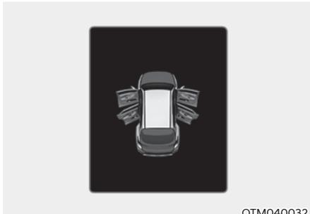
This warning is displayed if any door or hood or liftgate is left open. The warning will indicate which door is open in the display.
