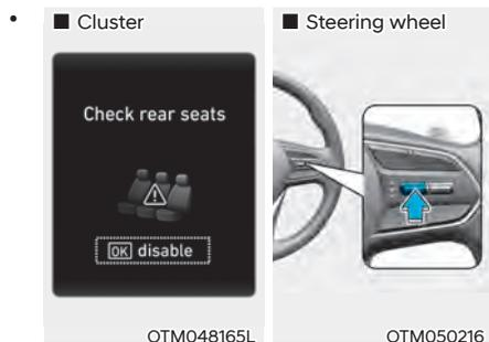
If you do not want to use Rear Occupant Alert, press the OK button on the steering wheel when the first alert is displayed on the cluster. Doing so will deactivate the second alert one time.
