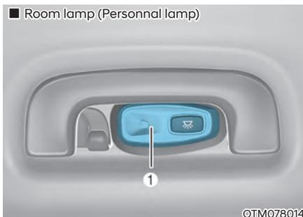
If the map lamp (LED/Bulb) (1) and the room lamp (LED type) (1) do not operate, we recommend that the system be checked by an authorized HYUNDAI dealer.
