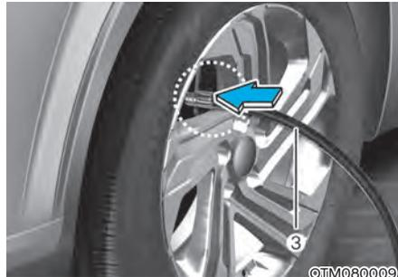
2. Connect the connection hose (3) of the compressor and tire into the tire valve.
