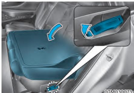
4. Pull on the seatback folding lever (2nd row seat), then fold the seat toward the front of the vehicle. When you return the seatback to its upright position, always be sure it has locked into position by pushing on the top of the seatback.
