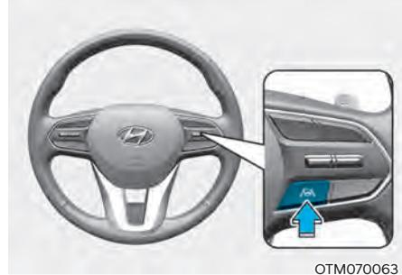
With the engine on, press and hold the Lane Driving Assist button located on the steering wheel to turn on Lane Keeping Assist. The white
