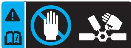
The electric motor for the cooling fan may continue to operate or start up when the engine is not running and can cause serious injury. Keep hands, clothing and tools away from the rotating fan blades of the cooling fan.
