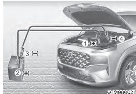
5. Connect the jumper cables in the exact sequence shown in the illustration. First connect one jumper cable to the red, positive (+) jumper terminal of your vehicle (1).
