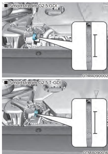
6. Pull the dipstick out again and check the level. The level should be between F (Full) and L (Low).
