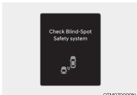
When Blind-Spot Safety system is not working properly, the 'Check Blind-Spot Safety system(s)' warning message will appear on the cluster, and the system will turn off automatically or the system will be limited. We recommend that the system be inspected by an authorized HYUNDAI dealer.
