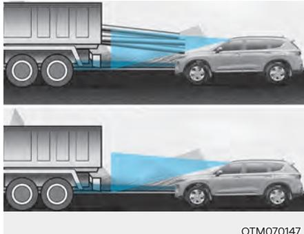
In the following cases, the vehicle in front cannot be detected by the sensor:
