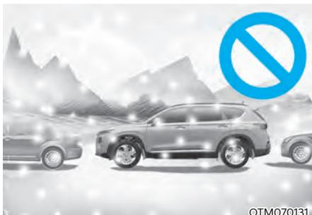
Snow may interfere with sensor operation, or Remote Smart Parking Assist may cancel if the road is slippery while parking.
