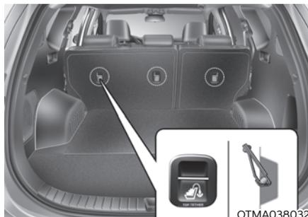
First secure the child restraint with the LATCH lower anchors or the seat belt. If the child restraint manufacturer recommends that the top tether strap be attached, attach and tighten the top tether strap to the top tether strap anchor.
