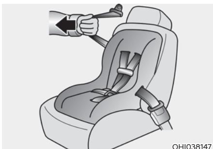
3. Pull the shoulder portion of the seat belt all the way out. When the shoulder portion of the seat belt is fully extended, it will shift the retractor to the "Automatic Locking" (child restraint) mode.
