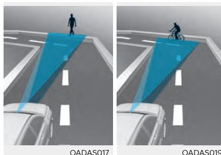
Forward Collision-Avoidance Assist may not detect other vehicles, pedestrians or cyclists in front of you on curved roads adversely affecting the performance of the sensors. This may result in no warning or braking assist when necessary.
