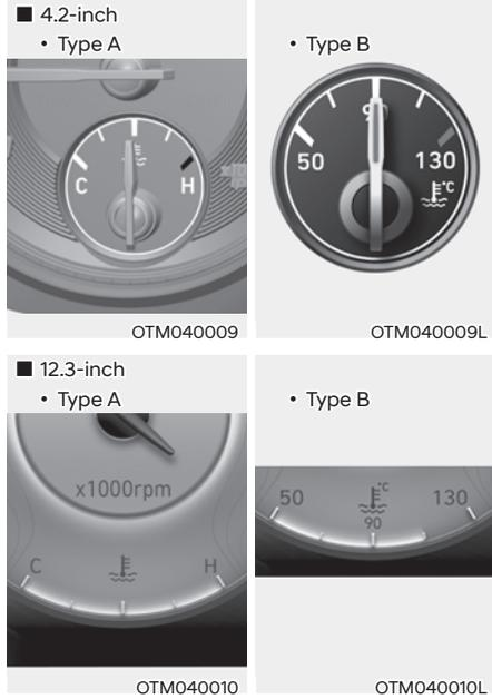
This gauge indicates the temperature of the engine coolant when the ignition switch is in the ON position.
